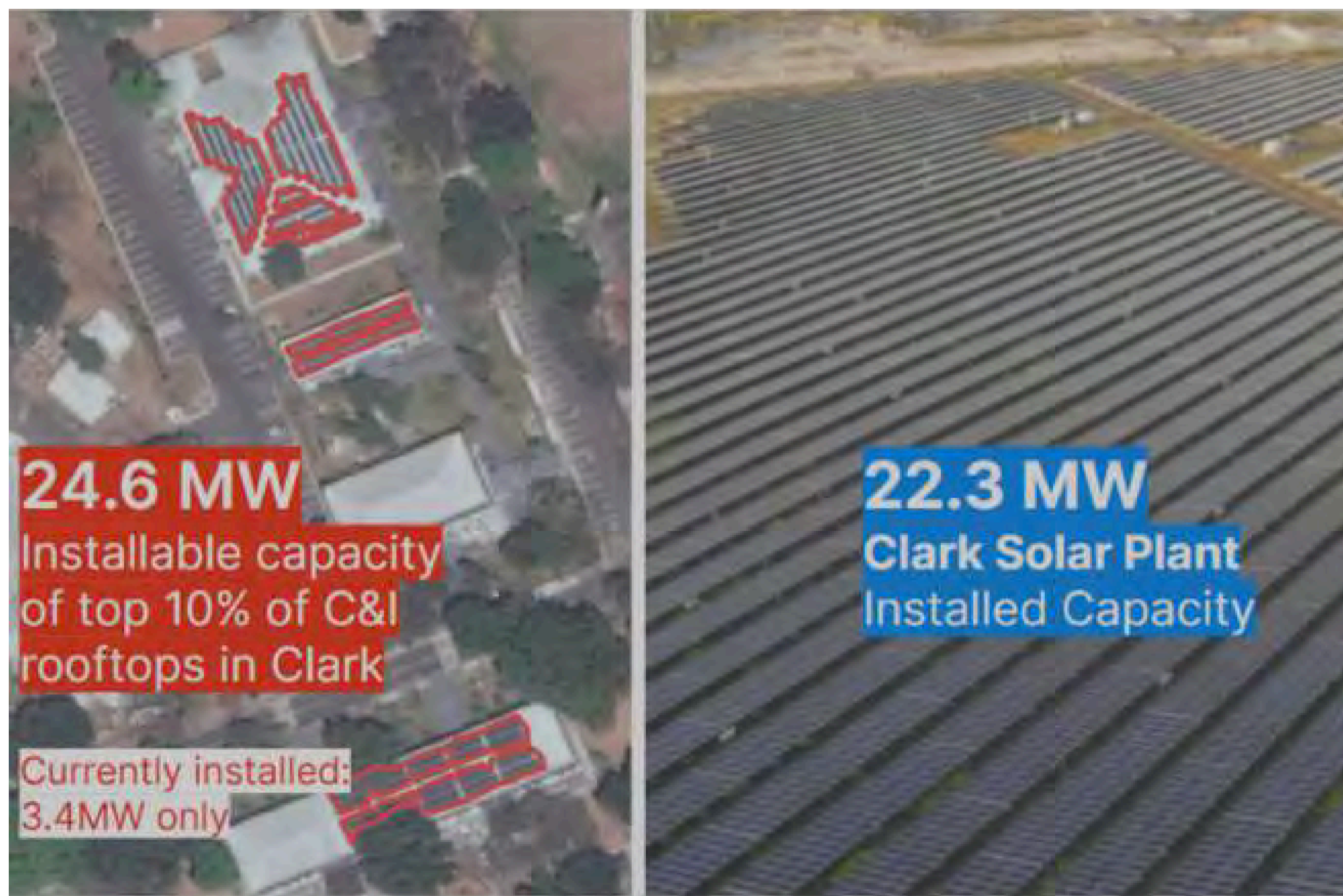
Figure 19. Installed Capacity of Top C&I Rooftop VS. Clark Solar Plant.
