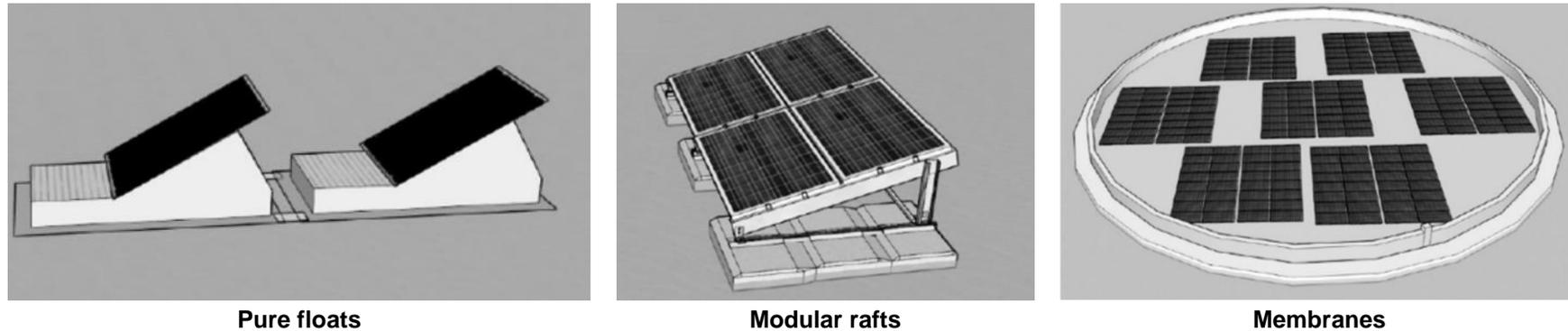
Source: MDPI Design and Analysis of a Floating Photovoltaic System for Offshore Installation: The Case Study of Lampedusa
